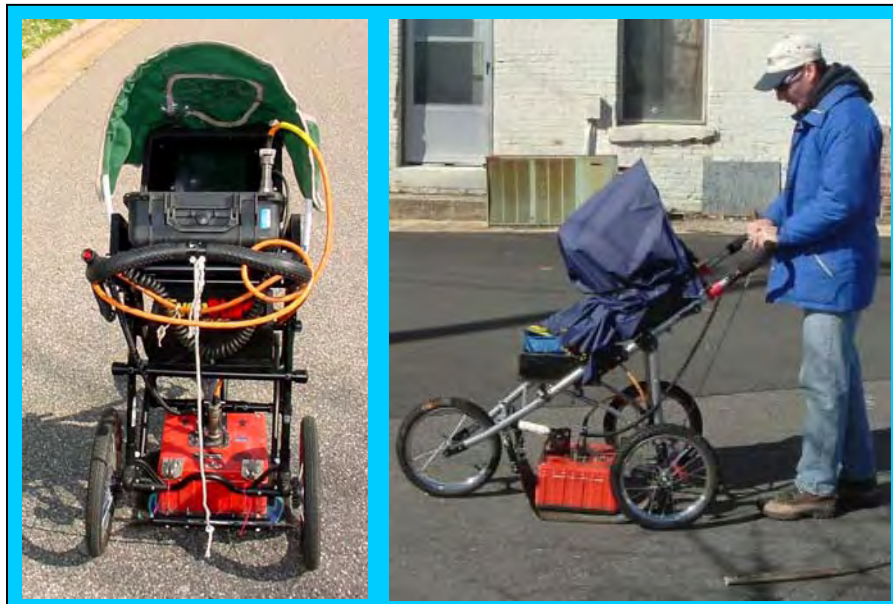
The photos show the SIR-2000 GPR system equipped with a 400 MHz antenna that were used to conduct the ground penetrating radar investigation at the Old South Main Street and East "A" Avenue sites in Salisbury, North Carolina on June 29 & July 7, 2006.
